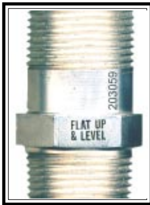
Flow Element Serial Number. Also Showing Sensor Orientation Flat. (Located near the enclosure. It is also on the enclosure tag.)
