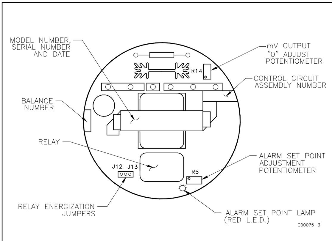
Figure 3-2. Control Circuit Outline Drawing
