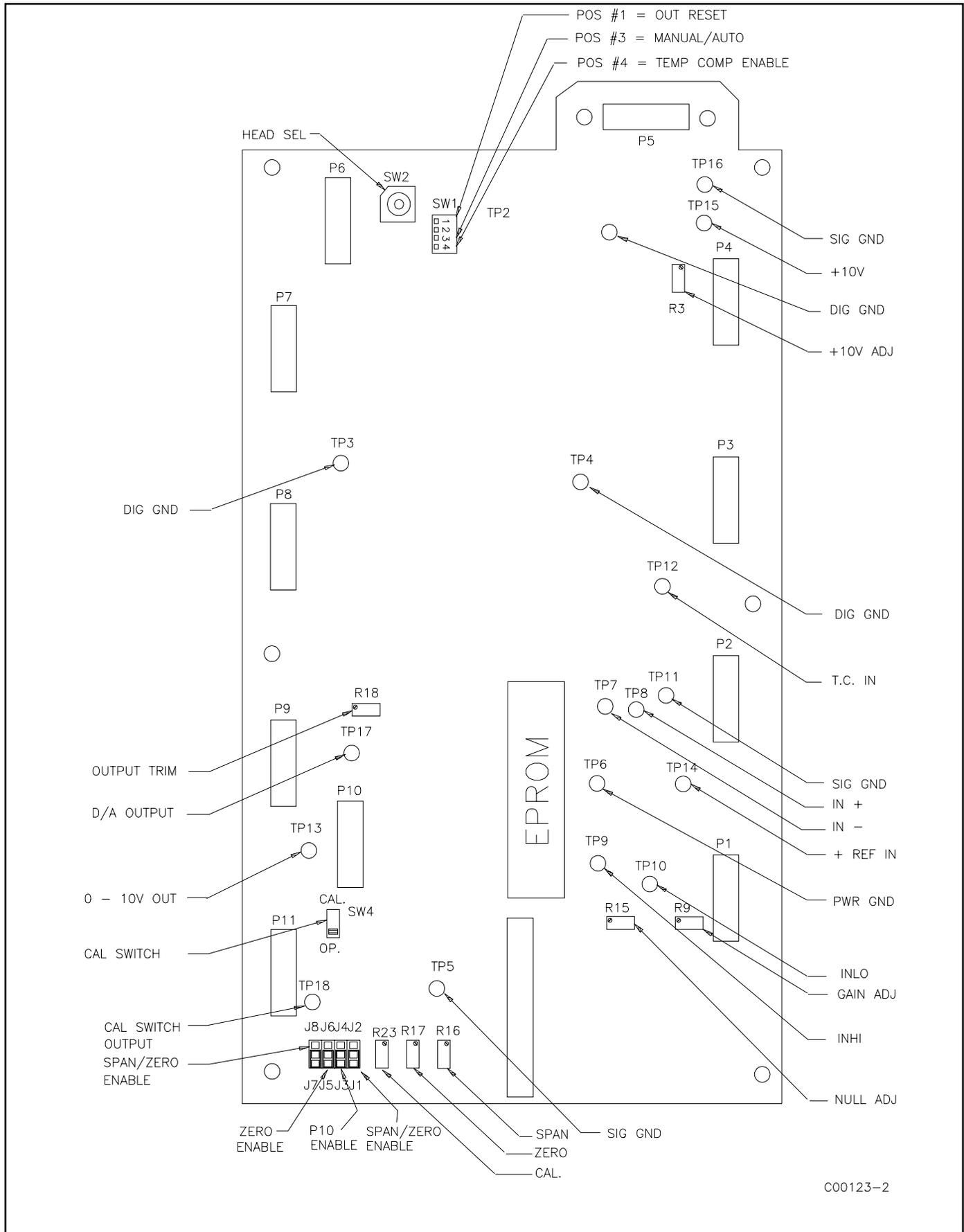
Figure 5-3. Control Board Layout
