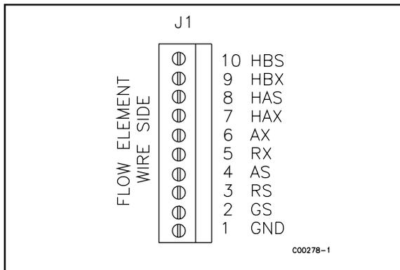
**Figure 5-1. J1 Connector Plug on the Backplane Board**
