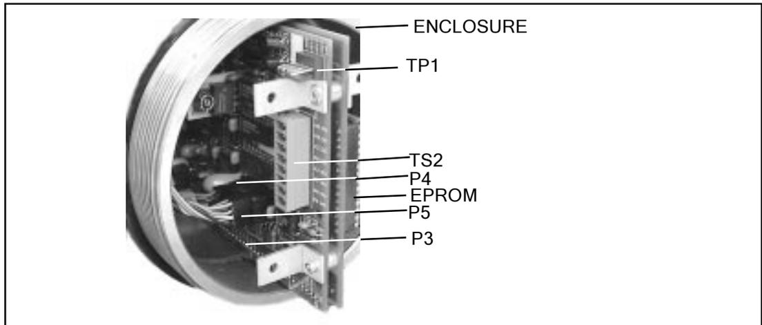
Figure 5-1. Component Identification
