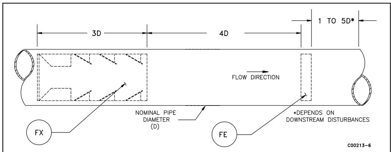
Figure 1-1. Typical Vortab Installation
